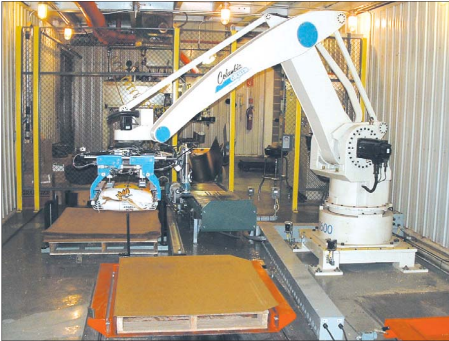
Renk Seed Company installed a Columbia/Okura LLC Model A1600 robotic palletizer in the same area where two workers had previously manually stacked bags of corn and soybean seed. A safety screen separates the packaging area from the palletizer. (Brett Renk phot)
