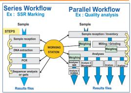
Management of sequences of analysis: management of flow type by series (all samples go from one work station to the next automatically) or in parallel (the user can choose whether or not to divide or group together the sample group manually),
